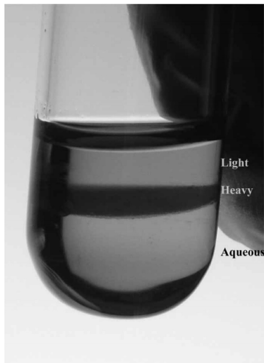
FIGURE 7 Formation of a third phase in 1.1 M, TBP/HPT solution. [65] HPT, hydro-genated polypropylene tetra-; TBP, tributyl phosphate.
