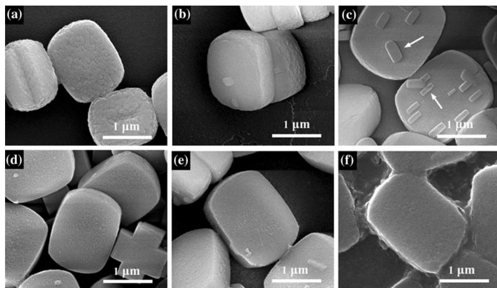
**Fig. 11** SEM images of MFI microcrystals after growth in secondary growth solutions not subjected to hydrothermal pretreatment. The secondary growth was initiated at 130 °C for (a) 1 h, (b) 2 h, and (c) 3 h, respectively; and MFI microcrystals after growth in secondary
