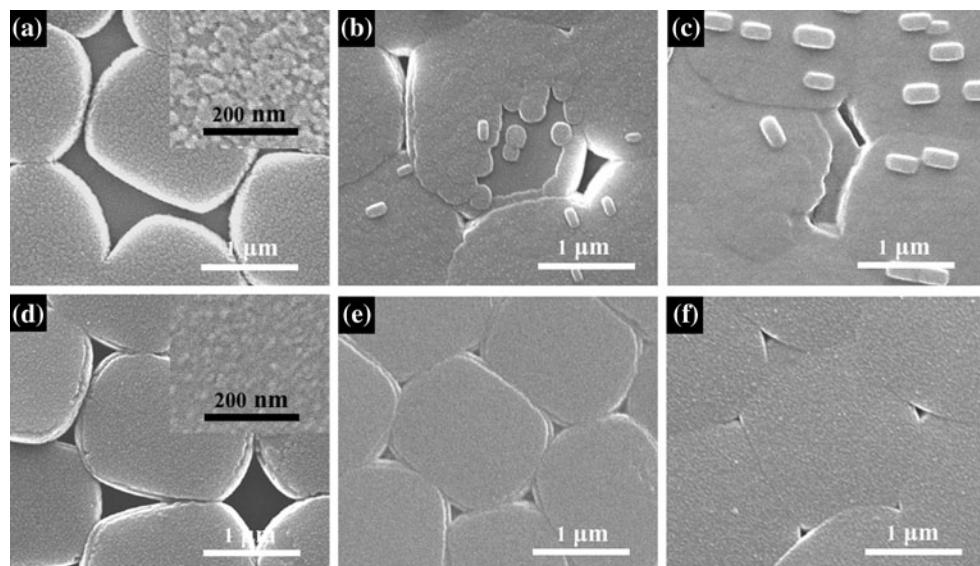
**Fig. 9** SEM images of MFI films synthesized in secondary growth solutions not subjected to hydrothermal pretreatment. The secondary growth was initiated at 130 °C for (a) 1 h, (b) 2 h, and (c) 3 h, respectively; the MFI films were synthesized in secondary growth
