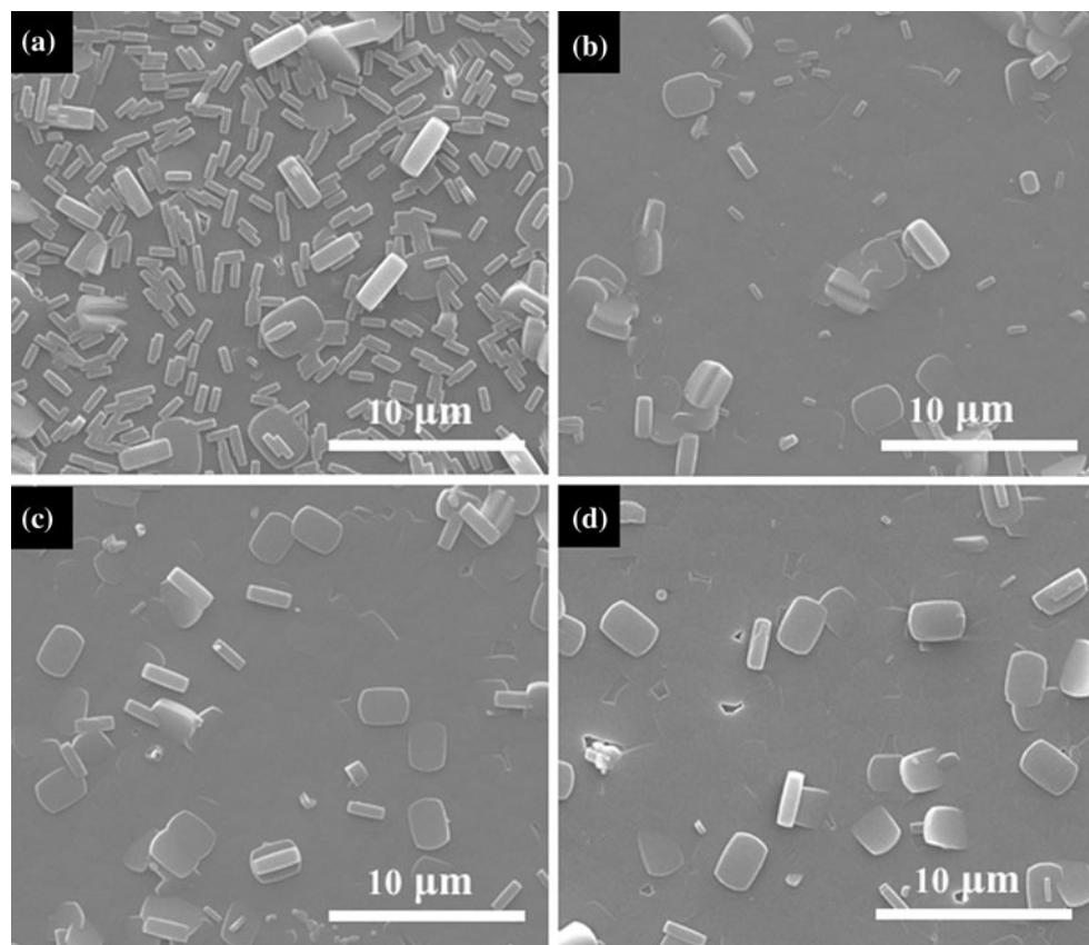
**Fig. 8** SEM images of MFI films synthesized in secondary growth solutions subjected to hydrothermal pretreatment at 150 °C with durations of (a) 0.5 h, (b) 1 h, (c) 5 h, and (d) 12 h. The secondary growth was initiated at 150 °C for 3 h
