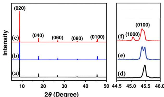
**Fig. 4** XRD patterns of the MFI films synthesized in the secondary growth solution subject to hydrothermal pretreatment at 150 °C for 2 h. The secondary growth was maintained at (a) 130 °C, (b) 150 °C, and (c) 170 °C for 5 h with  $2\theta$  at 5°–50°; (d), (e), and (f) are enlarged images. Note: prepared MFI films were not calcined before XRD characterization
