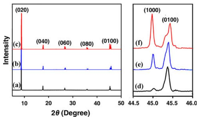
**Fig. 6** XRD patterns of MFI films synthesized in secondary growth solutions not subjected to hydrothermal pretreatment. The secondary growth was maintained at (a) 130 °C, (b) 150 °C, and (c) 170 °C for 5 h with  $2\theta$  at 5°–50°; (d), (e), and (f) are enlarged images. Note: prepared MFI films were not calcined before XRD characterization
