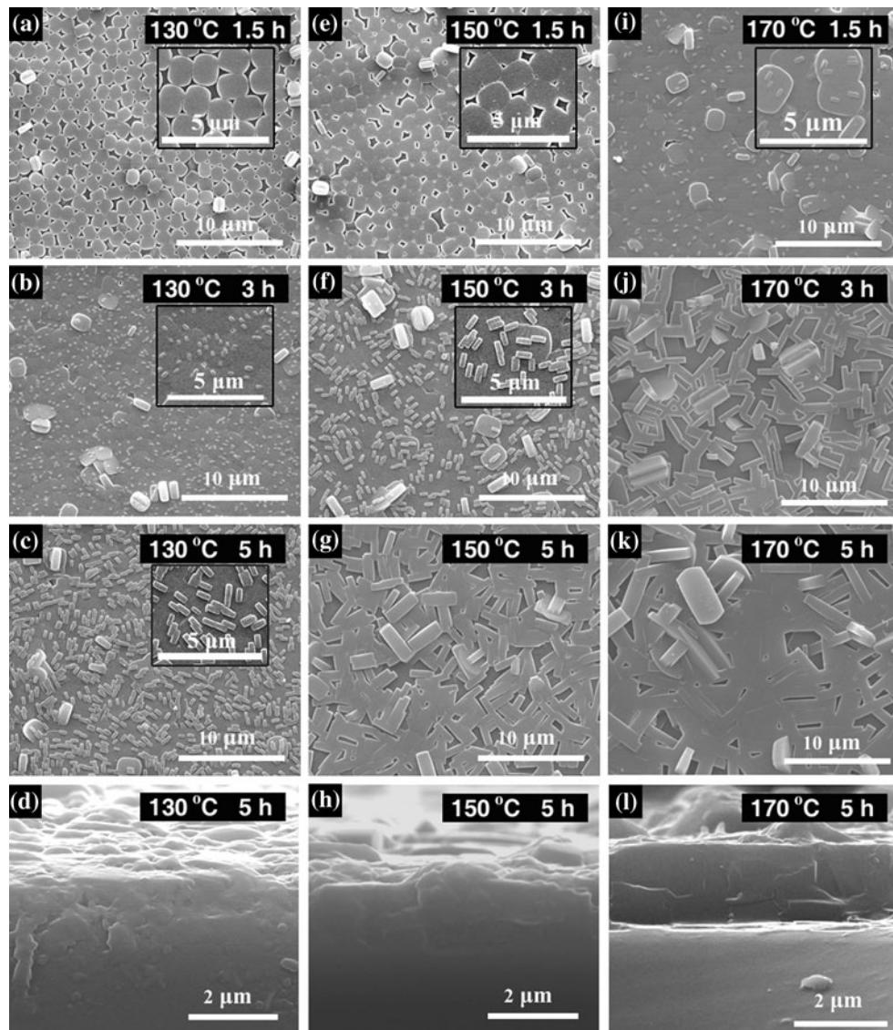
**Fig. 5** SEM images of MFI films synthesized in secondary growth solutions not subjected to hydrothermal pretreatment. The secondary growth was initiated at **a–d** 130 °C, **e–h** 150 °C, and **i–l** 170 °C for 1.5, 3, and 5 h, respectively
