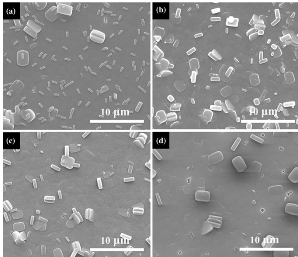
**Fig. 7** SEM images of MFI films synthesized in secondary growth solutions subjected to hydrothermal pretreatment at (a) 110 °C, (b) 130 °C, (c) 170 °C, and (d) 185 °C with the duration of 2 h. The secondary growth was initiated at 150 °C for 3 h
