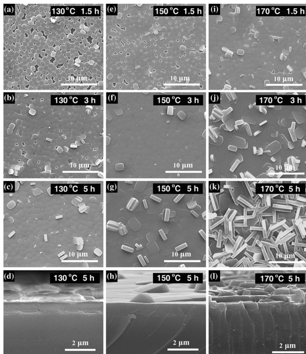
**Fig. 3** SEM images of MFI films synthesized in secondary growth solutions subject to hydrothermal pretreatment at 150 °C for 2 h. The secondary growth was initiated at **a–d** 130 °C, **e–h** 150 °C, and **i–l** 170 °C for 1.5, 3, and 5 h, respectively
