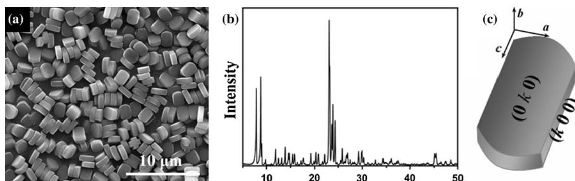
**Fig. 2** **a** SEM image of prepared MFI microcrystals, and **b** XRD pattern of the MFI seeds, and **c** schematic illustration of the detailed morphological features of MFI microcrystals
