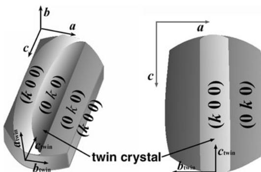
**Fig. 1** Schematic illustration of the relevant crystal planes and directions on MFI twin crystal
