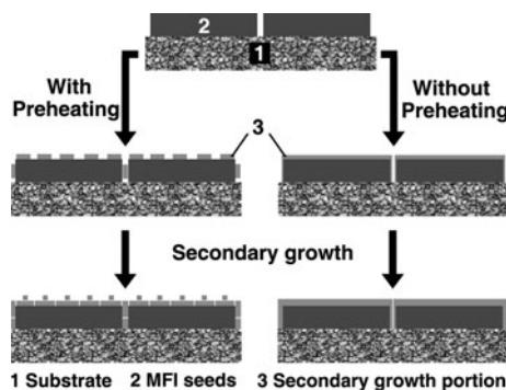
**Fig. 10** Illustration of the growth mechanism of *b*-oriented MFI monolayers during secondary growth with the precursor solution subjected to and/or not subject to hydrothermal pretreatment
